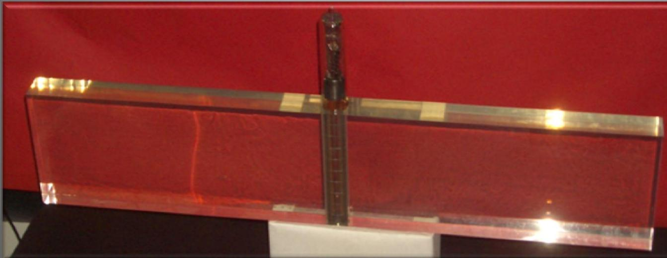
Photo of scintillator of  $50 \times 200 \times 1000 \text{mm}^3$  with the PMT FEU KF introduced inside the scintillator body.
