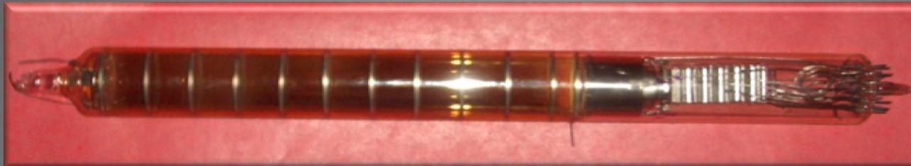
Photo PMT (PMT FEU KF) with sizes of photocathode  $\text{Ø}40 \times 200 \text{mm}^2$ , evaporated aluminum corbels are intended for leveling electric potential along the photocathode.
